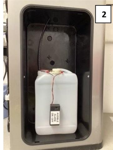
The alarm will silence once the overflow container has been emptied. Alternatively, you can switch it off manually using the switch attached to the overflow container.
